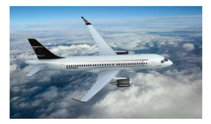
The CSeries will be constructed of advanced composites (47%), aluminum lithium (23%), standard materials (22%) and titanium/steel (9%). AVIC I (China) has the contract to manufacture the center section of fuselage, doors, and tailcone; wings will be built by Bombardier at Belfast, Northern island; and the aft fuselage and cockpit will be constructed at Saint-Laurent, Quebec. Final assembly will take place at Montréal-Mirabel.
