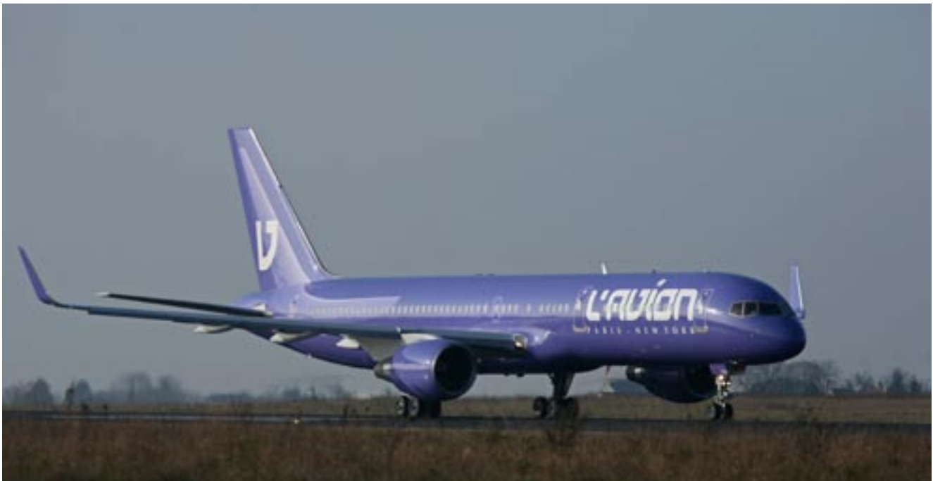
The 757-200, fitted with Aviation Partners Boeing winglets, was delivered to Orly on November 8, 2006.
