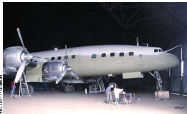
Restoration of the Connie began in 2001, and by February 2003 a coat of protective primer had been applied. Good progress was made once the aircraft was under cover.
